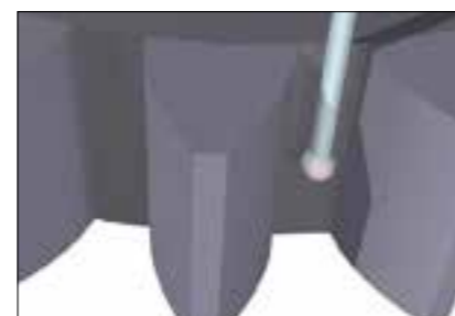
Measurement of microscopic gear tooth and tooth-form profile / tooth-alignment profile
