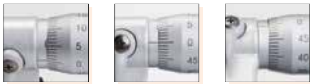
(a) From above the index line (b) Looking directly at the index line (c) From below the index line
