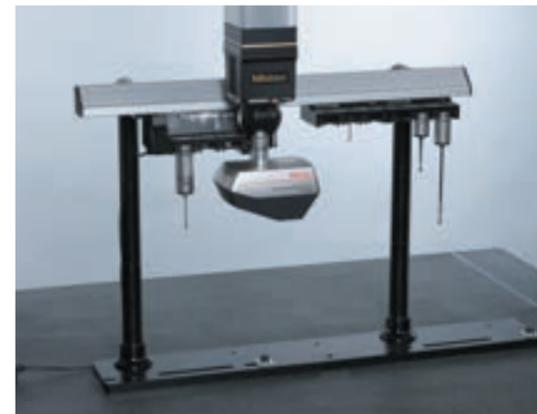
Note: Even after using the warm-up unit such as ACR3 (special order), it is necessary to warm up the laser for about 10 minutes.
