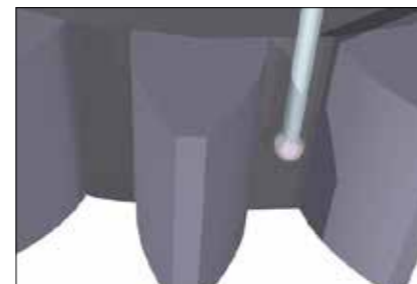
Measurement of microscopic gear tooth and tooth-form profile / tooth-alignment profile
