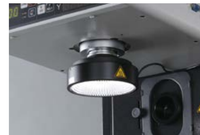
Example of attaching the LED circular illuminator on PJ-PLUS
