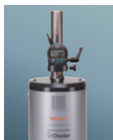
Inspection using digital type indicator
