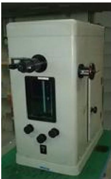
Figure 28 Koester interferometer (Interference Comparator made by Carl Zeiss Jena Corporation in former East Germany)
