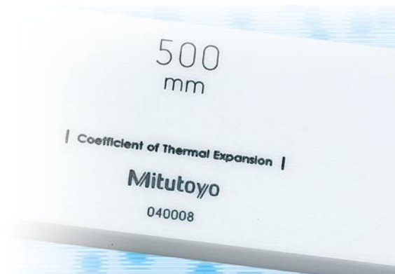
Figure 45 Gauge block with a calibrated coefficient of thermal expansion
