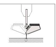
Using the universal holder allows easy hole centering. The dial face always faces upward when the indicator is rotated, which makes reading easy.
