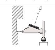
The dial face obliquely faces upward, allowing users to read the graduations from the user's side. It is convenient when probing on the side of a large workpiece and the workbench is high.
